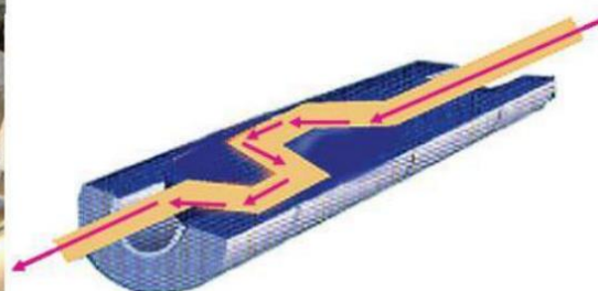
Fig.5. Microfluidizer M-110-EH and interaction chamber design diagram
