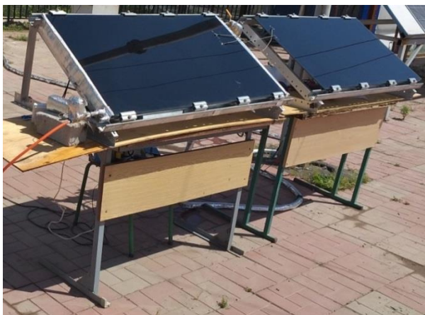
Fig.1. Photo of the experimental installation of the PVTI and PVM
