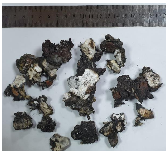
Fig. 5. Solid slag formed at a temperature in the combustion zone of 900-1000 ° C
