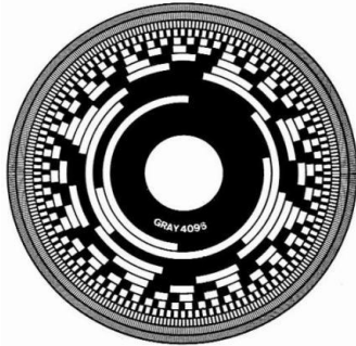
Fig.2. General view of the encoding disc gray code and binary code.
