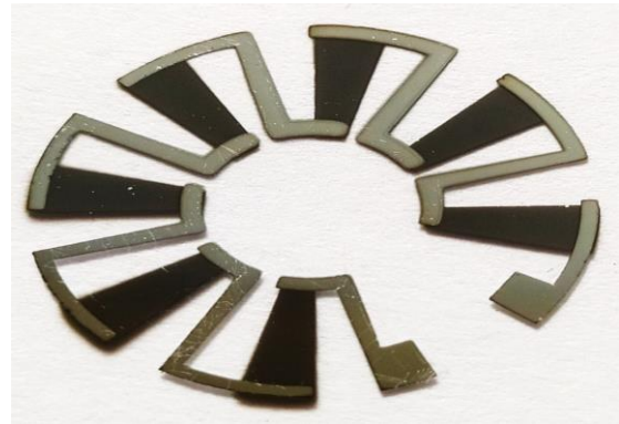
Fig. 9. Sputtered CoSi side of the device in the form of a camomile.
