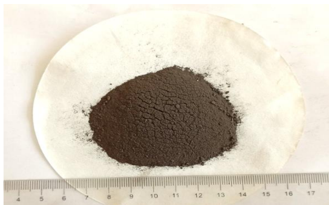
Fig.3. The magnetic fraction of the product formed after the sintering of zinc cake with crushed technical sulphur
