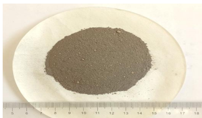
Fig.2. A sample of a charge made from a mixture of samples of zinc cake and technical sulphur
