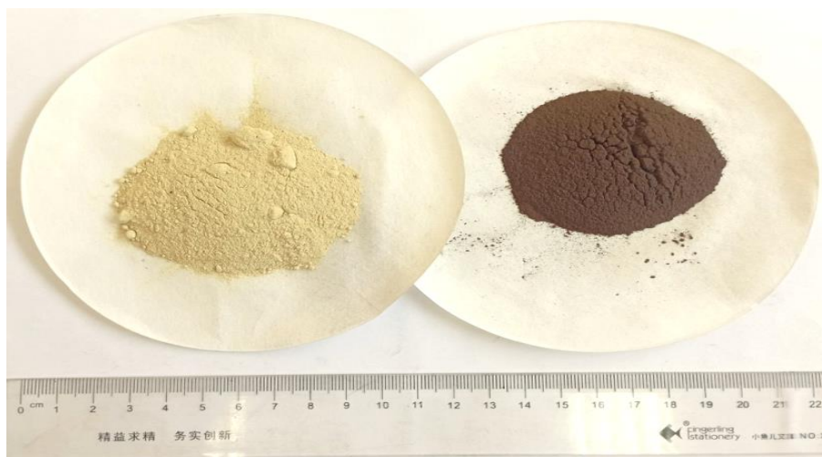
Fig.1. Granulometric analysis of a sample of zinc cake (right) and crushed industrial sulfur (left)
