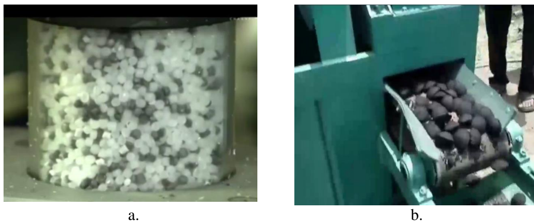
Figure 2. Waste treatment of polyethylene bags: a - granulation, b - carbonation in a special furnace
