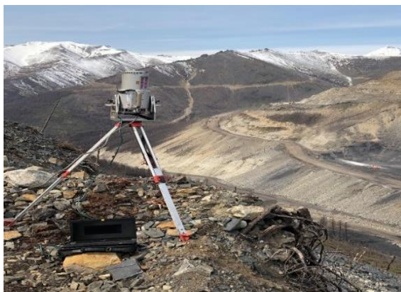
Fig. 2. Installation on the operating point of the RIEGL Z-400I scanner
