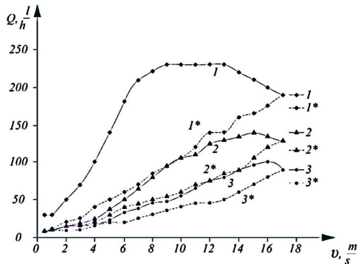
**Fig. 2.** The dependence of the specific permeability ( $Q$ ) of the F-1 membrane on the linear velocity ( $v$ ) of electrolyte 1, 2, 3 — increase in overpressure from 0.05 to 2.6 MPa 1\*, 2\*, 3\* — decrease in overpressure from 2.6 to 0.05 MPa
