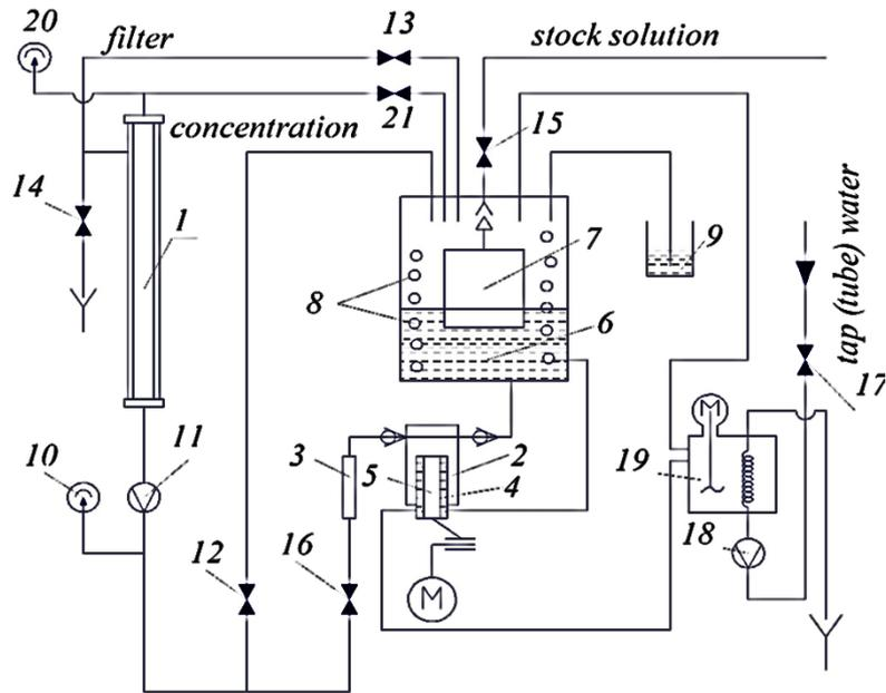
**Fig. 1.** Schematic diagram of the ultrafiltration unit 1 – ultrafilter with insert, 2 – pressure pump ND-0.4, 3 – accumulator, 4 – water jacket, 5 – plunger, 6 – recirculation vessel – storage, 7 – float system, 8 – coil, 9 – water lock, 10 and 20 – pressure gauges, 11 and 18 – rotameters, 12 ÷ 17, 21 – valves, 19 – thermostat.
