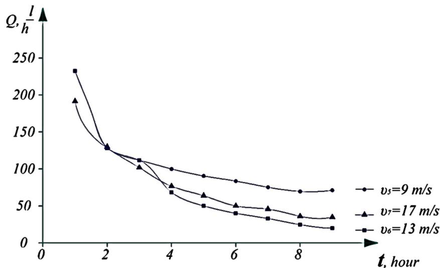
**Fig. 3.** The dependence of the specific permeability ( $Q$ ) of the  $F-1$  membrane on time ( $t$ ) at various linear velocities ( $V$ ): a) 1-3.0; 2-4.0; 3-5.0; 4-7.0; b) 5-9.0; 6-13.0; 7-17.0
