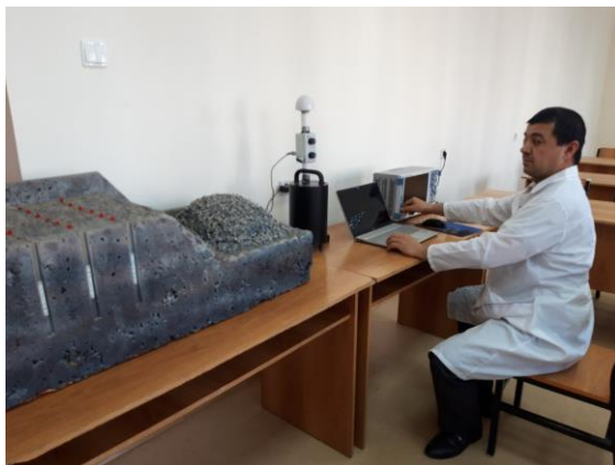
Fig. 2. Experimental studies of the action of stress waves in laboratory conditions
