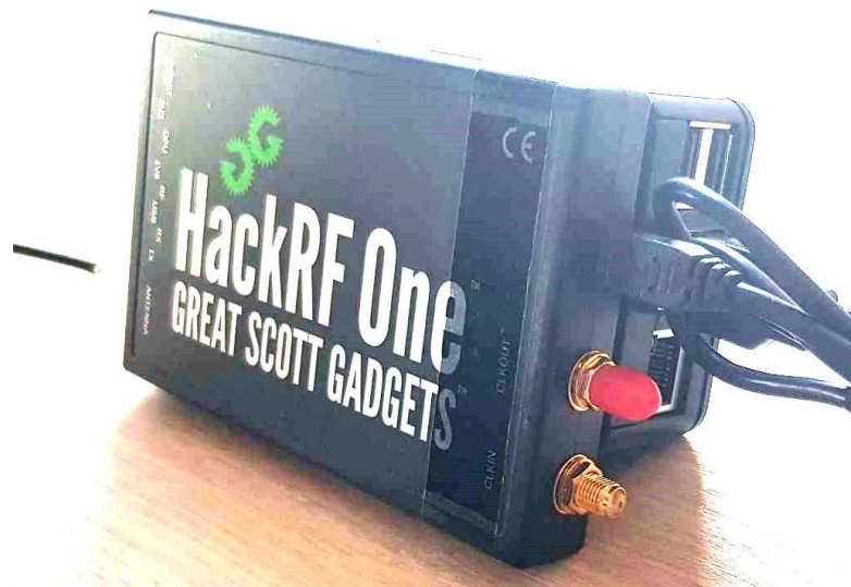
Fig. 1. Experimental setup with portable spoofer.
