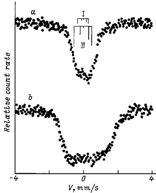
**Fig.2. Mossbauer emission spectra of  $^{61}\text{Cu}$  ( $^{61}\text{Ni}$ ) at 4.2K for  $\text{YBa}_2\text{Cu}_{2.8}\text{Fe}_{0.2}\text{O}_{7.03}$  (a) and  $\text{YBa}_2\text{Cu}_{2.5}\text{Fe}_{0.5}\text{O}_{7.18}$  (b) ceramics. For spectrum a, the position of the multiplets components corresponding to centers  $^{61}\text{Ni}^{2+}$  in nodes Cu (1) (I) and Cu (2) (II) is indicated.**
