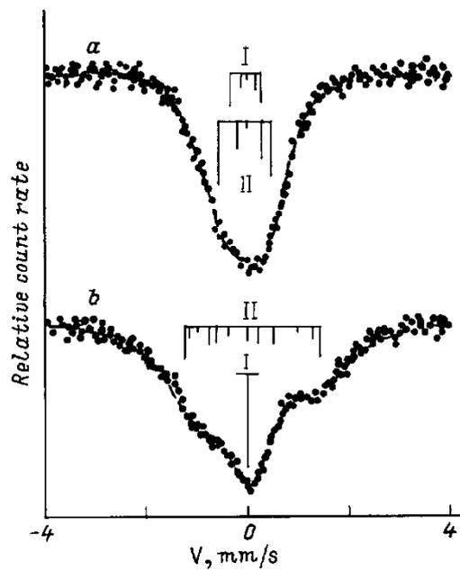
**Fig.1. Mossbauer emission spectra of  $^{61}\text{Cu}$  ( $^{61}\text{Ni}$ ) at 80 K for  $\text{YBa}_2\text{Cu}_3\text{O}_{6.96}$  (a) and  $\text{YBa}_2\text{Cu}_3\text{O}_{6.1}$  (b) ceramics. The position of multiplets components corresponding to  $^{61}\text{Ni}^{2+}$  centers in Cu (1) (I) and Cu (2) (II) nodes is indicated.**
